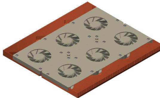
Fig. 3. Cooling system unit consisting of ultra-flat blowers and high fin number copper heat sinks; two cooling units are placed on opposite upright/vertical faces of the system.
