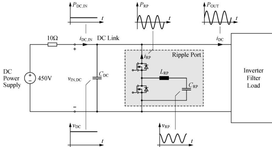
Fig. 2. Topology of the employed Ripple Port including schematic visualization of power flows and capacitor voltages.
