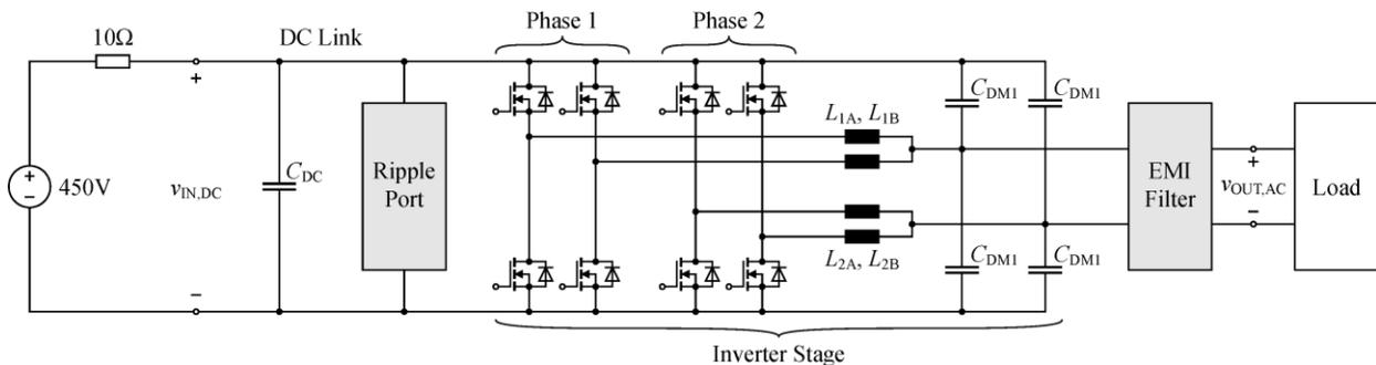
Fig. 1. Topology of the presented inverter consisting of two output phases, each of which is formed by two interleaved bridge legs in buck-configuration. The system DC-side energy storage (Ripple Port) is detailed in Fig. 2 and the EMI filter is presented in Fig. 4.
