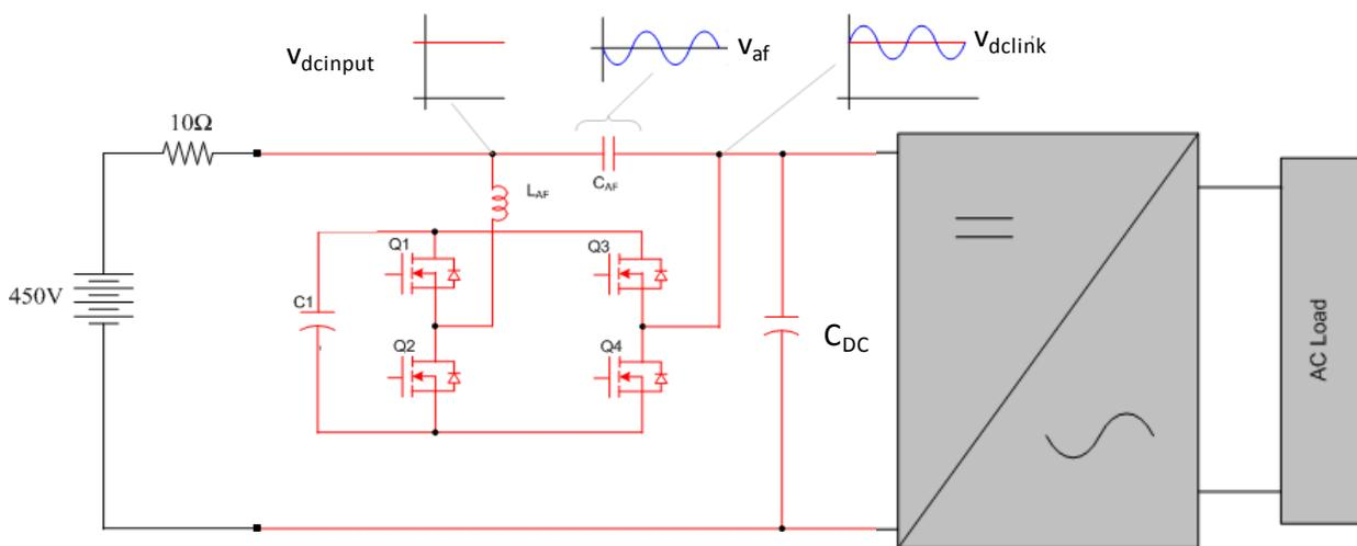
$C_{DC}$  : DC link capacitor (implemented: 400  $\mu$ F, 450V).
