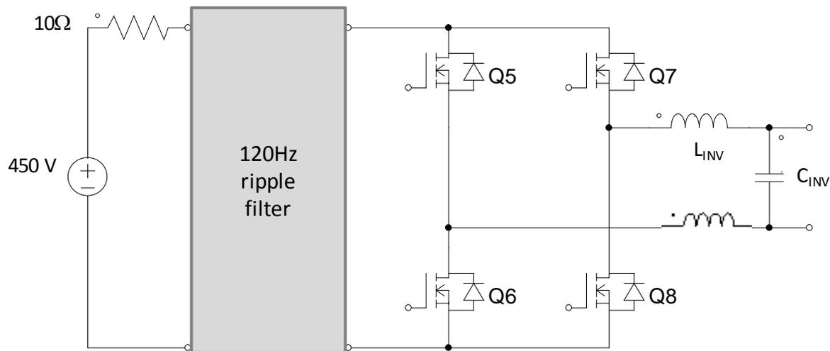
$Q_5 - Q_8$ : SiC MOSFETs, switching at 45 kHz.
