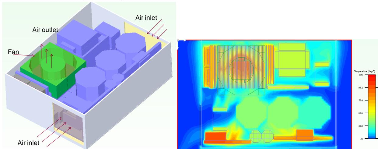
Fig. 4: (a) Cooling implementation (b) simulated temperature profile
