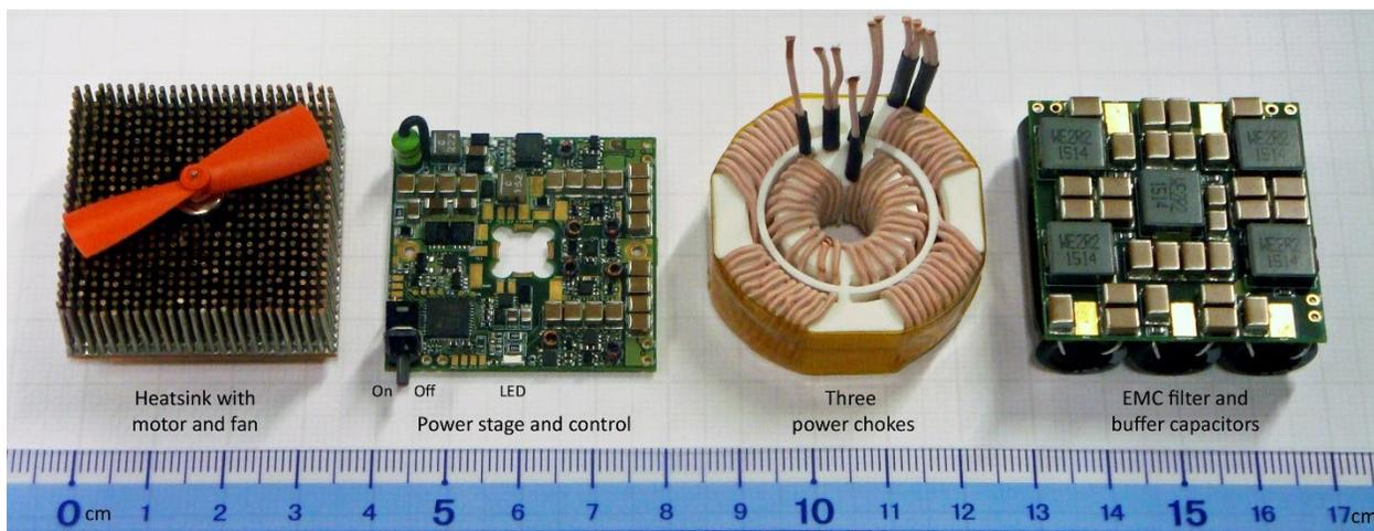
**Figure 2:** Photo of main sub-assemblies before final assembly (on 5 mm paper)
