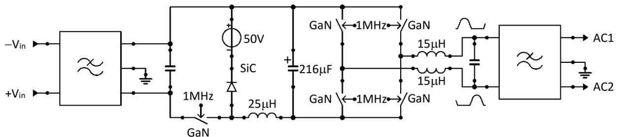
Figure 1: Inverter principle
